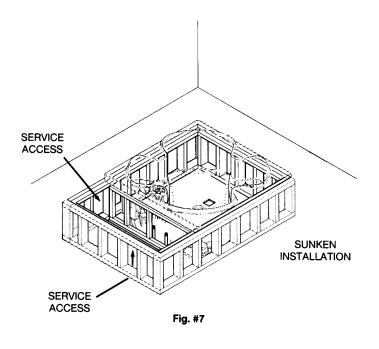
DO NOT SUPPORT THE WHIRLPOOL BY ITS RIM ONLY. PROVIDE SUPPORT WHEREVER POSSIBLE UNDER THE RIM TO PREVENT SHIFTING. ALL OF THE WEIGHT OF THE UNIT MUST REST ON THE BOTTOM PADS IN THE BASIN AREA.
